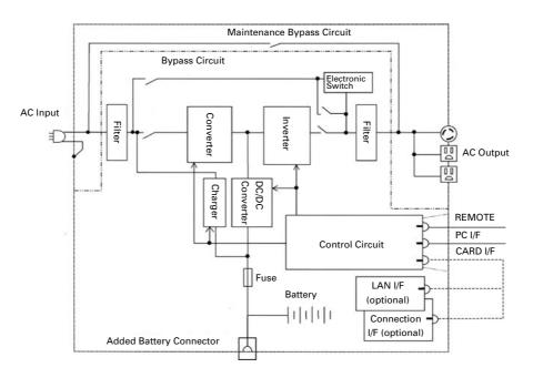
Fig. 4: Circuit Block Diagram
